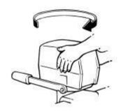
3. Move the gear shift lever quickly and firmly from neutral to forward.
