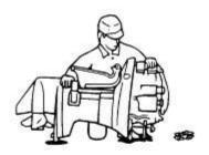
3. Drain the fuel from the carburetor, fuel filter, and fuel line.
